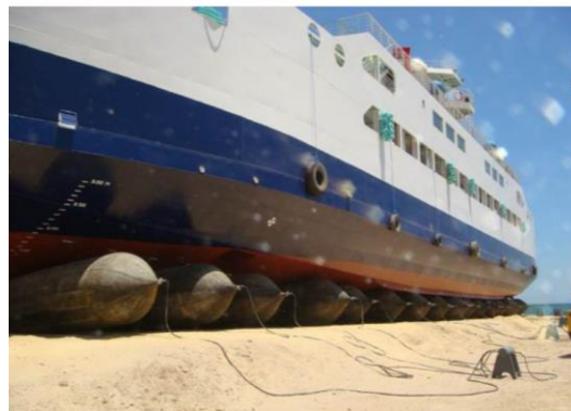
Fig. 11 – Ship launch using rubber airbags [7]
